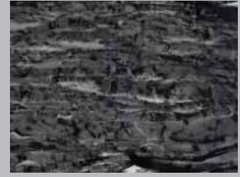
TEM of a cross-section of GEOMET®
