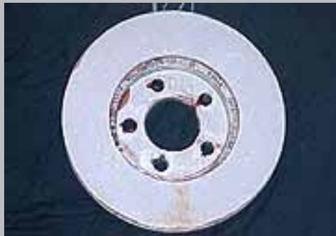
Heated to 662°F (350°C) prior to 60 cycles of SAE J2334, 14.6 microns
