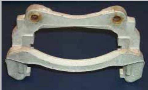
GEOMET® L 10 cycles of APGE. Uncoated internal threads were waxed before testing.
