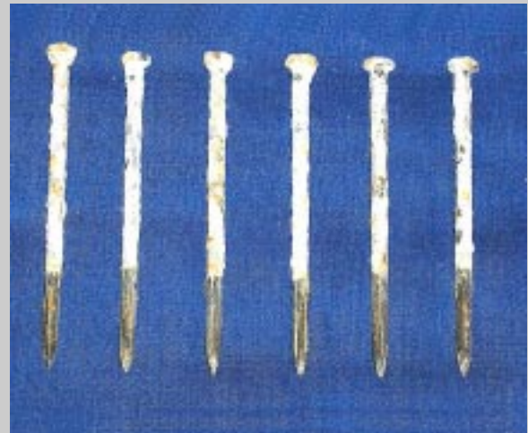
Hot Dipped tested in ACQ wood for 1000 hours SST
