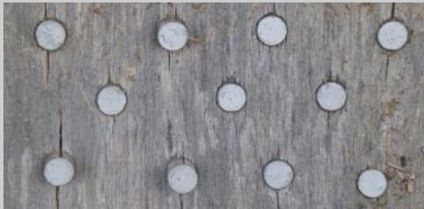
DACROMET® LTX in ACQ wood after one year outdoor exposure
