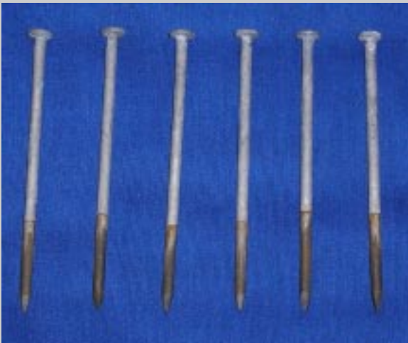
DACROMET® LTX tested in ACQ wood for 1000 hours SST
