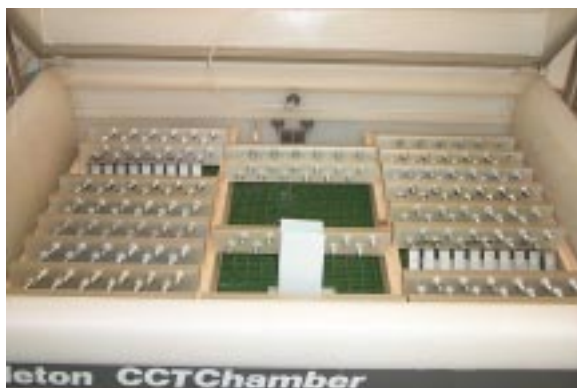
Fasteners installed in aluminum bars are mounted in Singleton CCT chamber for corrosion testing to GM 9540P
