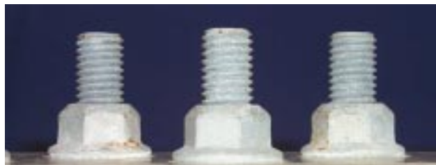
Prevailing Torque nuts coated with GEOMET® L at 120 cycles GM 9540P
