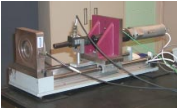
Labmaster 9504 used for torque-tension testing
