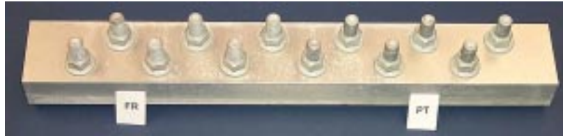
Prevailing Torque and Free Running nuts coated with DACROMET 500® B at 120 Cycles GM 9540P
