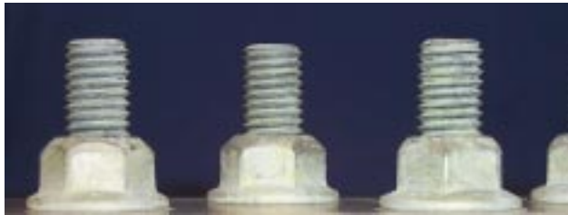
Prevailing Torque nuts coated with DACROMET 500® B at 120 cycles GM 9540P
