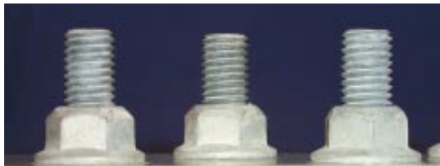
Prevailing Torque nuts coated with DACROMET 320® L at 120 cycles GM 9540P
