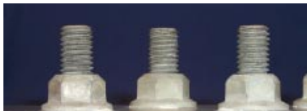
Prevailing Torque nuts coated with Cadmium + Yellow at 120 cycles GM 9540P
