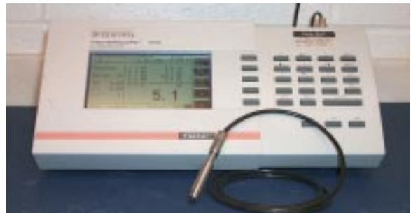
Fischerscope instrument used for thickness testing
